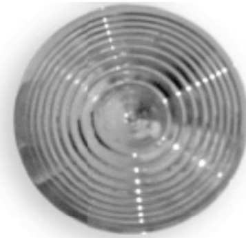
Figure 1: Diamagnetic Lens. The acoustic Fresnel lens is obtained by smoothing an acoustic lens of a convex one. This allows bringing high-resolution acoustic signals and focusing the energy at a specific depth. Fresnel’s lenses are formed by a set of concentric rings with decreasing width and each ring is called the “Fresnel region”. Between two consecutive regions, there is a \pi -phase difference. The main energy contribution to the focus is given by the central regions of the lens.
